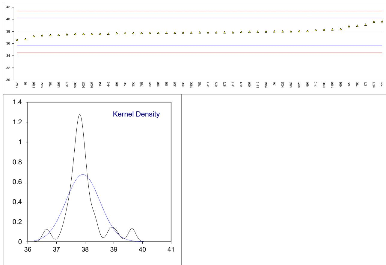
Determination of Kinematic Viscosity at 100 °C on sample #23250; results in mm<sup>2</sup>/s
