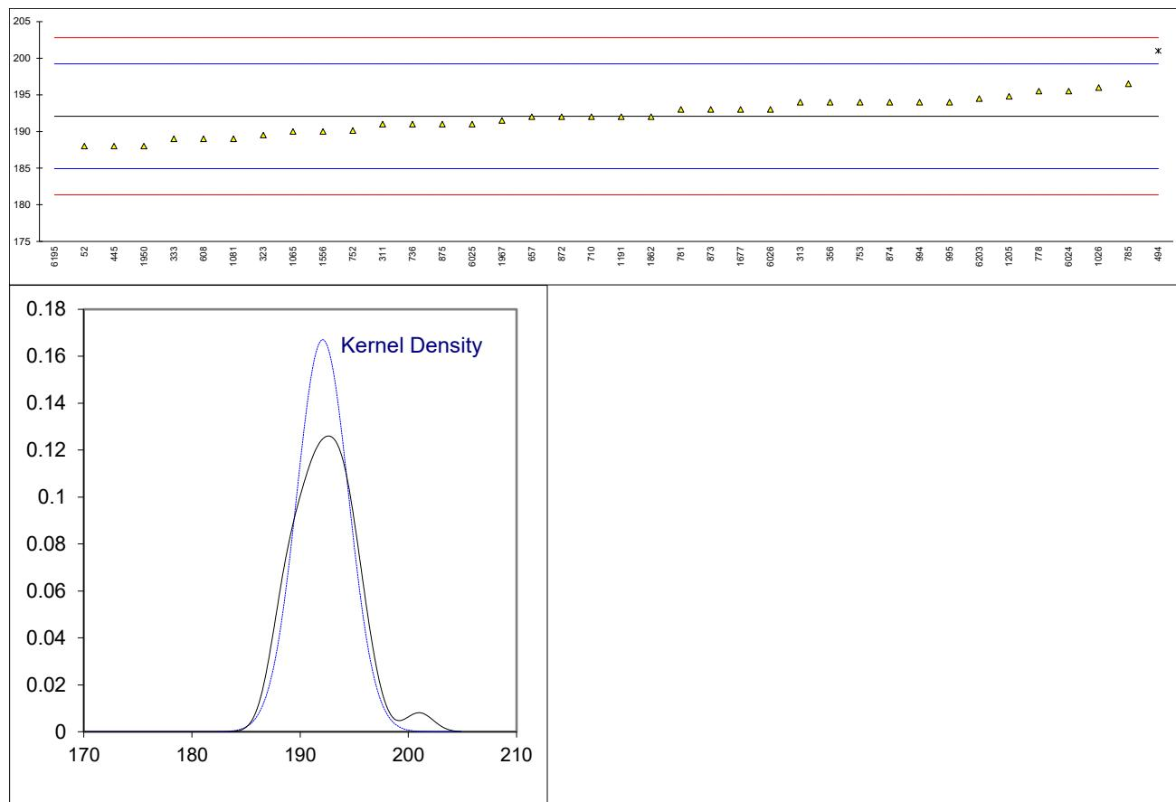
Determination of Kinematic Viscosity at 50 °C on sample #23250; results in mm<sup>2</sup>/s
